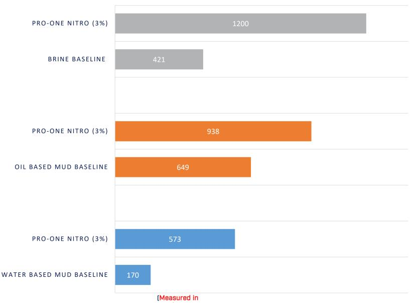
• Inch pounds is a measure of the amount of torque, and resultant heat and friction the lubricant can accept before breaking down
